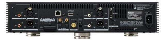
Around back the 701N is busier, with balanced (XLR) and unbalanced (RCA) inputs and outputs, paired optical and coax S/PDIF digital inputs, and both USB-B (streaming) and -A (drive) ports (another mini-USB port, for firmware updates, is marked "Software." There's also a wired-Ethernet network port, of course, plus an RS-232 serial port for a system controller, 12v trigger in/out minijacks, and a Bluetooth antenna bump-out.
