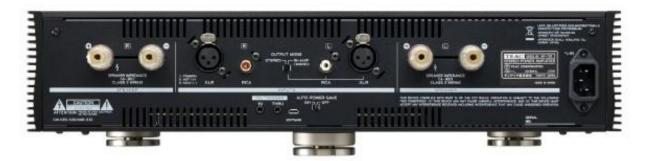
The rear panel presents a spaced pair of heavy, "WBT-type" banana/5-way jacks for each channel, a balanced (XLR-female) and unbalanced input (RCA) ditto, 12v-trigger in and through minijacks, and an IEC power-cord receptacle. A mini-USB port is labeled "Software" (though it's hard to imagine what software update a power amplifier might need), and mini-slide switches labeled Output Mode Stereo/Biamp, and Auto Power Save On/Off complete the facilities.
